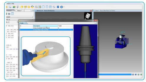
For accessibility within the machining area, safe tool changes, and checking the engagement conditions at the machining point, precise models of the tools are required.
