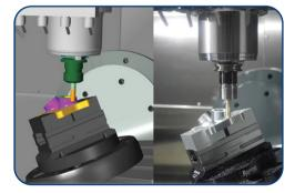
Easily download a 3D digital twin of your tool for NC verification. You can download data and specifications for many different CAM systems and even export to industry standards such as ISO13399/GTC, DIN4000. Source.
